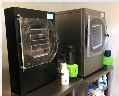
THE TWO FREEZE DRYERS THAT PULL THE LIQUID FROM FOODS MAKING THE PRESERVED WITHOUT HAVING TO ADD ANY INGREDIENTS FOR PRESERVATION .
